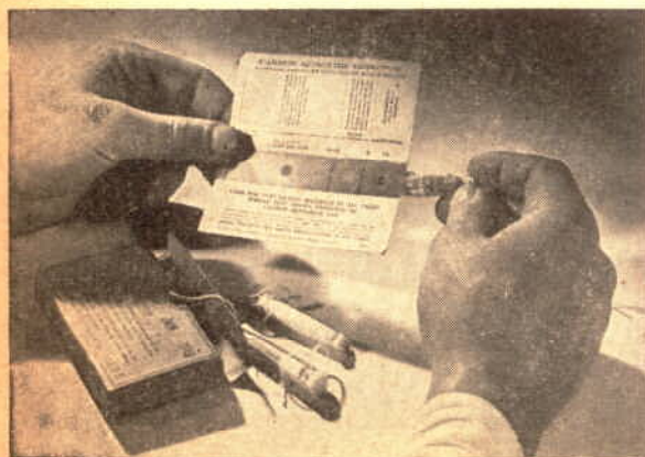
If monoxide is present, the detector will change color, the final color depending on the gas concentration. Comparing the exposed detector with a chart shows the concentration.
