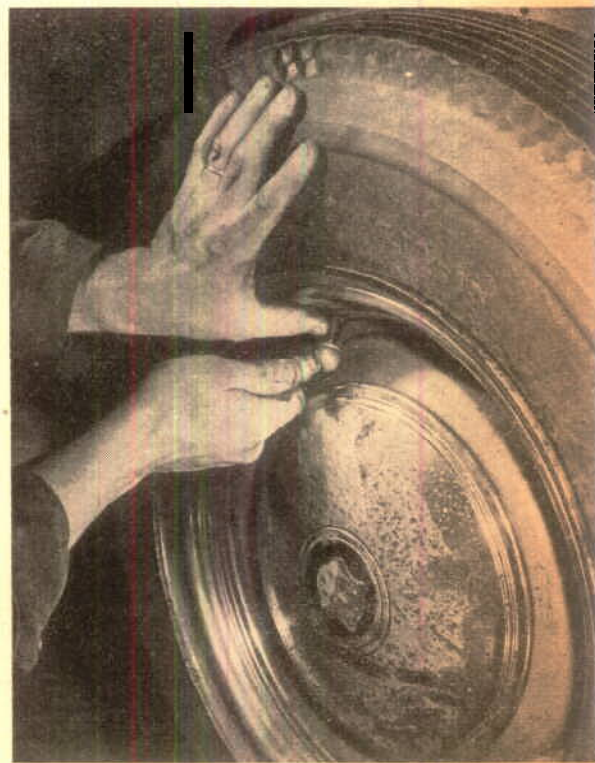
7. Pry on back bead. A tire iron quickly slips the inside bead over the rim after the valve stem has been lined up. When bead is on, the mechanic starts the stem through its hole.
