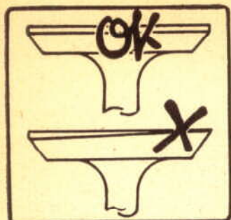
To be ground successfully, valves need a definite margin. A knife edge causes breakage and burning
