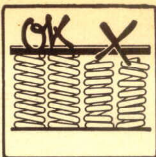
Use one new spring, if possible, when checking length and tension with the aid of a straightedge
