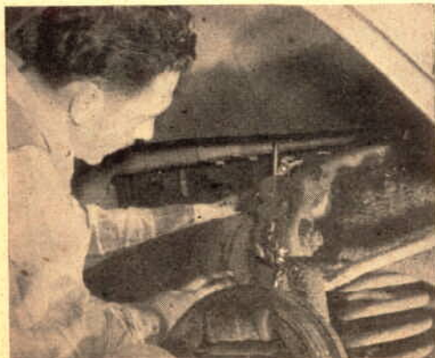
5. To reach the valves, the front is jacked up and the right wheel removed. Then the mechanic takes off the fender plate, heat shield, fuel line, and (above) side plates over the valves.
