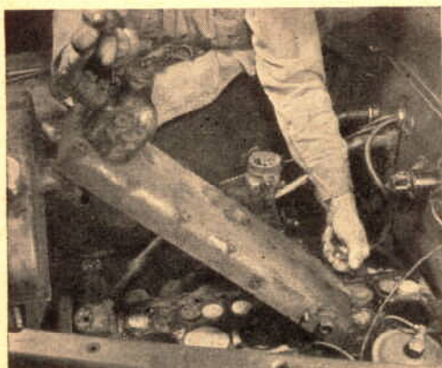
3. As the head is lifted off for cleaning, carbon may be seen on the piston and valve heads. The mechanic gets a good grip on the head; even aluminum ones are awkward to handle.
