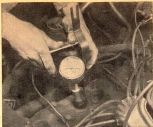
1. A compression gauge hints that the job is needed, as a low reading suggests that a valve is sticking or burned. In this shop, compression is always tested as part of a regular tune-up.
