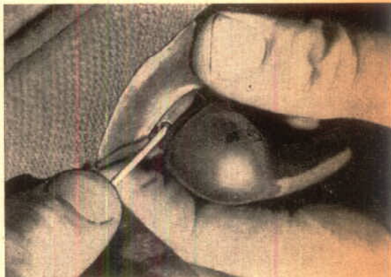
Take off door handle and window crank. Press inward on base plate to expose lock pin. Use small nail to push pin out of collar and shaft.
