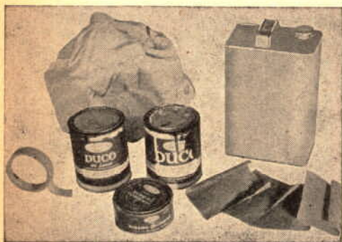
Refinishing the dent area requires thinner, primer-surfacer, rubbing compound, sandpaper, finishing color, and masking tape. Lacquer is preferable to enamel since it dries quickly.
