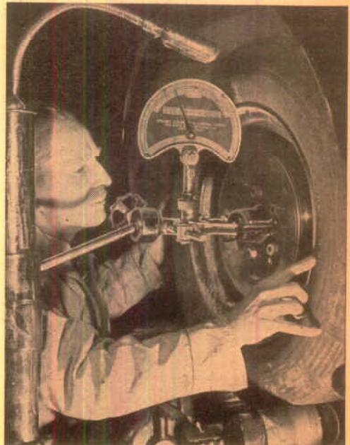
On a pre-vacation visit to your service station, have the wheels aligned. It is estimated that a tire \frac{1}{8} " out of line is dragged sideways 87' each mile, reducing life of the tire 20 to 50 percent.
