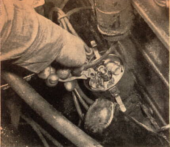
5. Contact points are removed from the distributor and cleaned with a fine-cut file. If the points are badly oxidized or pitted, new points and a new condenser are installed.
