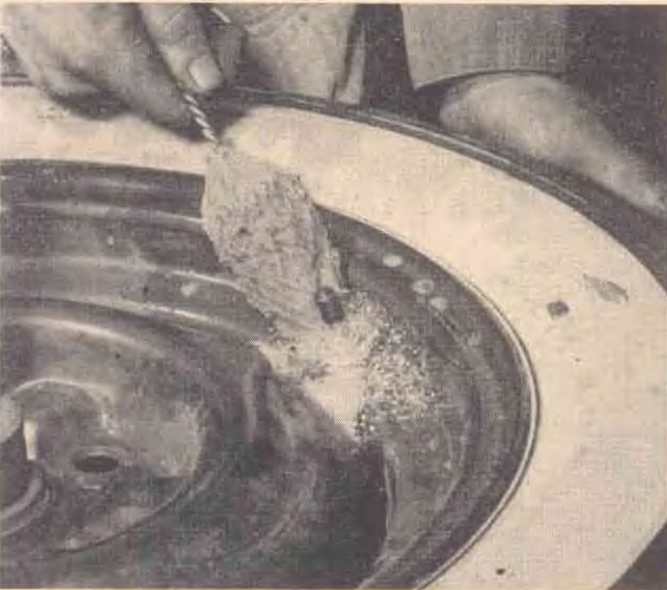
5 SOAPY WATER is used to check for leaks. Bubbles show that this valve is loose. Tightening it made the tubeless tire airtight.
