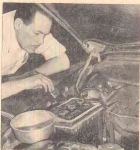
A CLEAN BATTERY with secure connections is first step in preventing an electrical breakdown in your car. Baking-soda-and-water paste will remove corrosion from terminals.
