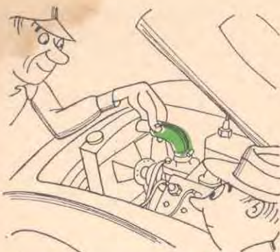
Spongy connections indicate hose decay
