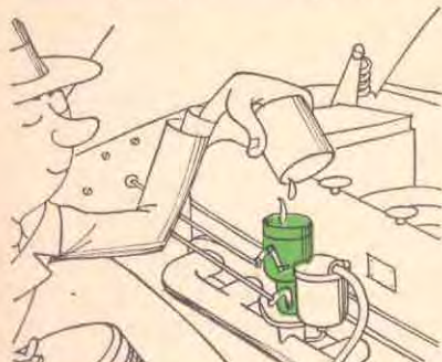
Direct action primes a parched carburetor
