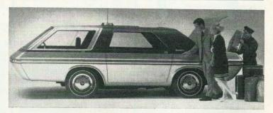
many other safety items. The car has a V-8 engine in front and conventional drive to the rear axle.
