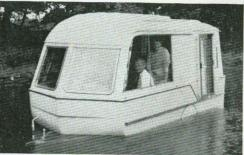
away under its own power-a seven-horse outboard. The hull is molded of fiberglass. On land, the 15-foot vehicle, with lounge and fully equipped kitchen, is easily towed by an average car to the next campsite.
