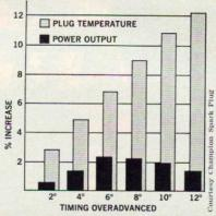
What happens when you power-time is shown graphically on this chart, made from dynamometer tests. Maximum power gain is two percent, with six degrees overadvance. Beyond that, the power falls off again, while the temperature of the plugs (and detonation) climb destructively.
