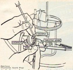
A dashpot slows the return of the throttle on some automatic-drive cars to prevent engine stalling. With the dashpot stem depressed, clearance between it and the lip of the throttle lever
