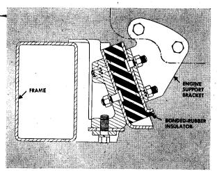
NEW SLANTING engine mountings insulate engine vibration from the frame better. Moreover, the rubber retains its elasticity. The car's roll center has been raised so that the body will lean toward the outside of a hard turn by 15 degrees less.
