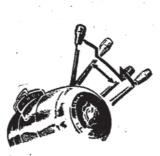
"NO-LOOKY" shift is fine for parking in tight quarters or rocking mired car: you just lift the lever a bit toward you and slap it up or down. If you don't lift, the gate restricts you to Neutral or Drive. As on other automatics, the starter works only in Neutral.
