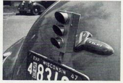
A THREE-COLOR Stop-N-Go Lite® for the rear of an automobile automatically tells the driver behind whether a car is traveling more than 10 miles an hour. A green light goes on when the car exceeds that speed. An amber light glows when brakes are applied, and a red one indicates speed is 10 m.p.h. or less. Made by Harrell Products, Milwaukee, the device has only two connecting wires and is easily installed.
