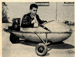
This three-wheeled vehicle combines a surplus airplane wing tank, a 1½-hp. gasoline water-pump engine, scooter wheels, and an airplane stick for steering. Robert Ferreira built it as a high-school shop project in Danville, Calif. A chain drive from the engine to the single rear wheel propels the scooter at speeds up to 30 m.p.h. The steering stick turns the vehicle in the direction that it's leaned. Vertical is straight ahead.
