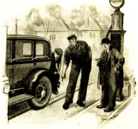
"Look at the tracks of your tires," Gus said. "The wheels are out of line. Either you sprung the frame when the wheel hit the curb or you moved the back axle on the spring."
