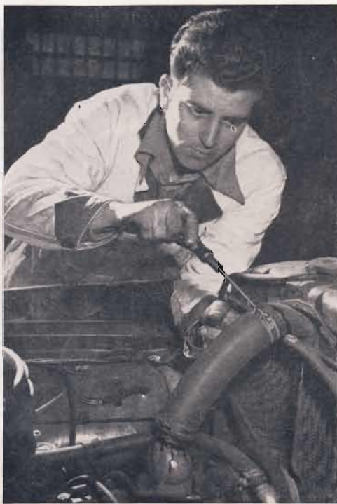
Radiator hoses are inspected and defective ones replaced. All hose clamps should be tightened carefully to prevent possible leakage of antifreeze solution
