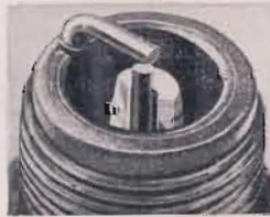
CRACKED AND BROKEN
