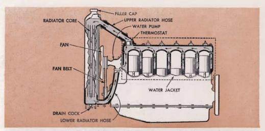
Water is circulated through the system when the engine is running and, os it passes through the woter jacket, absorbs heat which it carries to the radiator where it is dispersed into the air flowing through the radiator
