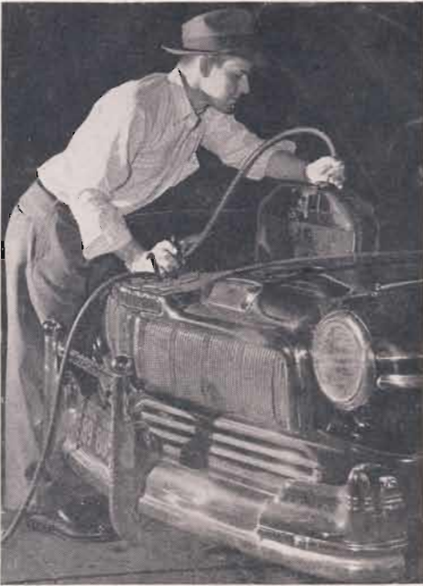
Radiators on many cars can be flushed with a garden hose after cleaning compound has had time to do its work. Hose at radiator outlet is disconnected
