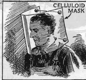
Fig. 1. How the face shield is made of a piece of celluloid.
