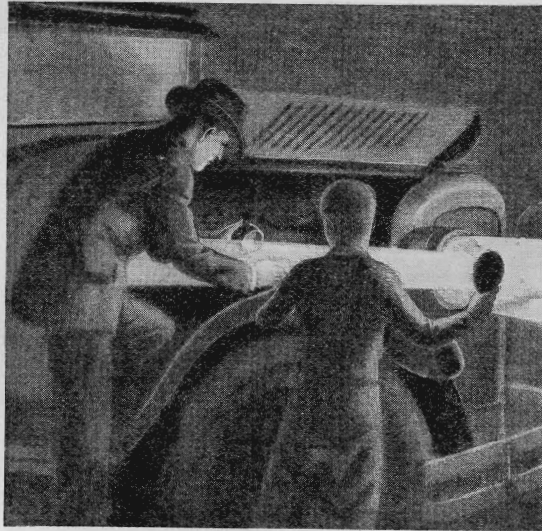
If you have no trouble light, one can be improvised by using a small hand mirror to reflect headlight beams.
