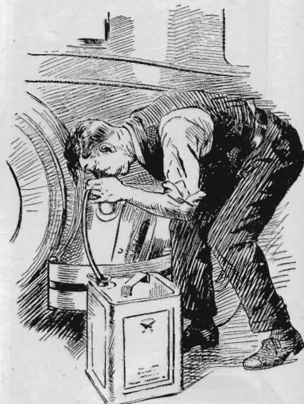
Fig. 4. Blowing into the auto gas tank forces gasoline through a siphon tube into a container.
