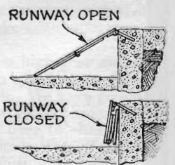
Fig. 4. Steel plates fastened together make a folding runway to take your car over the curb that stands between garage and street.
