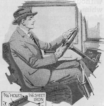
Figs. 1 and 2. A convenient arm rest for a closed car. Fig. 2 shows its simple construction at a glance
