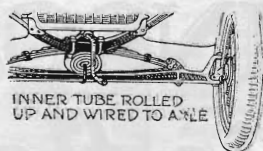
Fig. 8. A rolled-up inner tube will act as shock absorber if a spring should weaken
