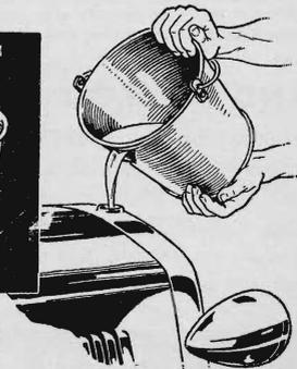
A spout cut in the pail keeps water from spilling on the finish of the car
