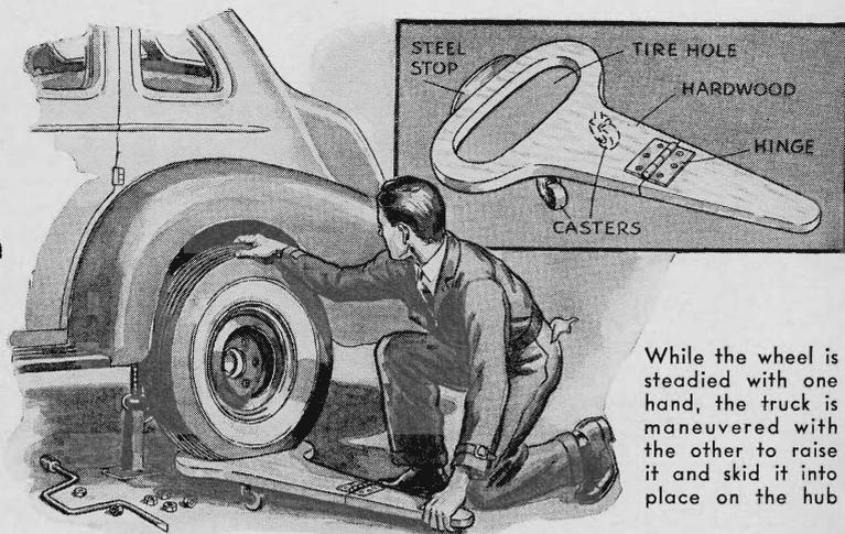
While the wheel is steadied with one hand, the truck is maneuvered with the other to raise it and skid it into place on the hub
