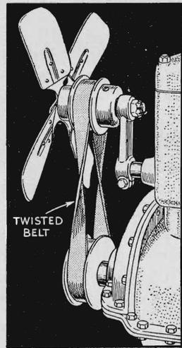
NOT long ago, I found that the motor of my car was running hot and finally traced the cause to a loose fan belt. When I tried to fix this, I discovered that the tension adjustment had been tightened to the limit. Being unable to replace the belt immediately with a new one, I found a solution to the problem by giving the flat belt a twist, as shown in the illustration reproduced at the left. This
