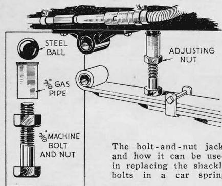
FROM an ordinary machine bolt and nut, a scrap of gas pipe, and a steel ball bearing, the amateur mechanic can provide himself with a powerful midget jack that will prove valuable for many types of repair jobs. As shown in the drawing, the jack is assembled by slipping the pipe over the end of the bolt and placing the ball bearing in the upper end of the pipe. To adjust the jack, it is necessary only to turn the nut with a wrench. A considerable amount of lifting power is obtained.—F. C.
