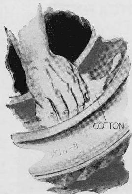
THE NEXT time you have difficulty locating the tack or nail that caused a punctured tire, rub a large wad of absorbent cotton around on the inner wall of the shoe. No matter how small the point of the nail or piece of metal may be, it will catch in the cotton and pull off a telltale tuft that will indicate its exact position in the inner wall of the shoe.—W. H.
