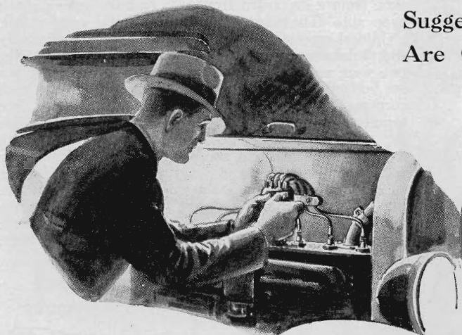
By installing a lamp fixture on the front of the dashboard, as shown in the circle, a light is provided for your work as indicated above
