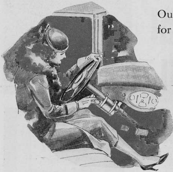
Holder made of radiator connection hose is attached to steering column and keeps your flashlight always handy
