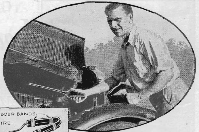
Two old magnets from a Ford fitted with extensions, as shown at left, can be used to pick up small parts dropped into inaccessible places around the motor as illustrated above
