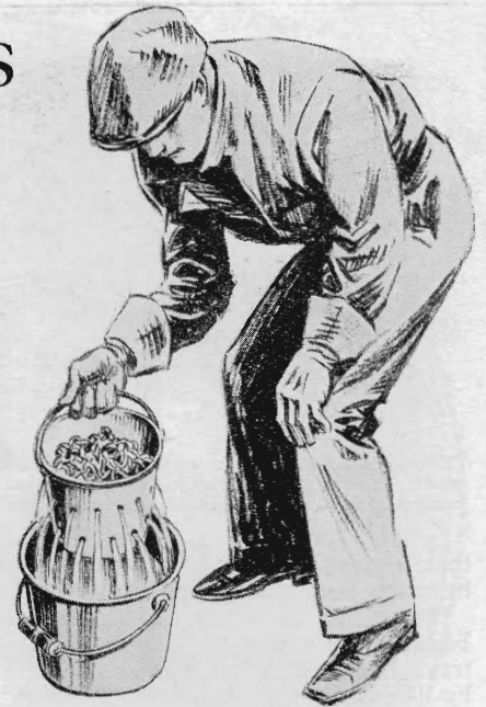
Fig. 5. Big pail and perforated small pail make handy apparatus for washing mud from chains
