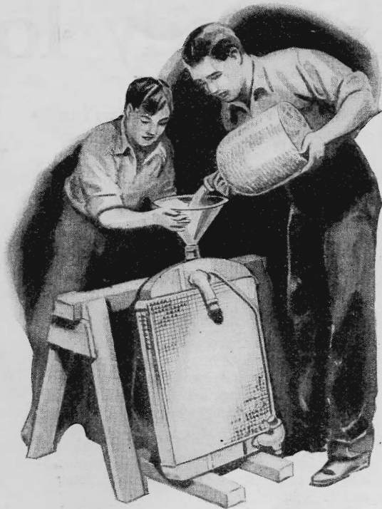
A heavy scale in radiator may be removed by ten percent solution of hydrochloric acid.
