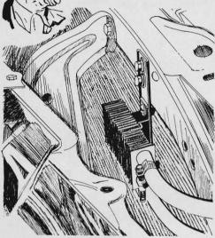
If fuel percolation is a problem, you can correct it by installing a cooler between the fuel pump and carburetor. Use the \$3.85 power-steering cooler from a 1966 Cadillac (part #1482078). Mount it in a spot where it will receive adequate flow of cool air.
