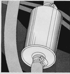
Cure clogging of small "in-carburetor" fuel filters by fitting a large, separate filter, such as General Motors' AC GF-61-P, in the fuel line. These filters are disposable, but have greater capacity and long life. Available from GM dealers and auto-supply stores.
