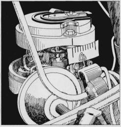
To check centrifugal advance on GM V-8 distributors, remove cap and mark rotor with a thin vertical line. Make a 7/64-inch scale (eight degrees between marks). Align rotor and scale at starting point, hand-turn to full advance, and read off the degrees.
