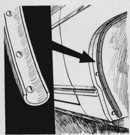
Reduce mud and slush runoff from the wheel wells with a length of soft ½-inch rubber or vinyl hose. Slit open the hose and secure it to the fender liner about 1½ inches back from the edge of the opening. The slit side of the hose, facing the wheel, works as a gutter.
