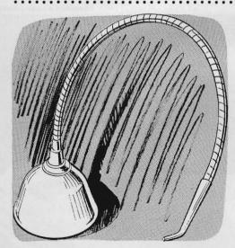
A flexible extension for your oil can is easy to make. Next time you replace a speedo cable hose, save a foot of it at the instrument end. Then cut the tip off an oil can and solder or cement one end of the hose to the neck, the other to the tip. Presto—a gooseneck oiler.
