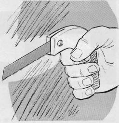
An old keyhole-saw handle can be fitted with a broken hacksaw blade to make a handy tool for undercutting the commutators of startermotor and generator armatures. Grind the blade as shown in the drawing, and insert it with the teeth pointed towards the handle.
