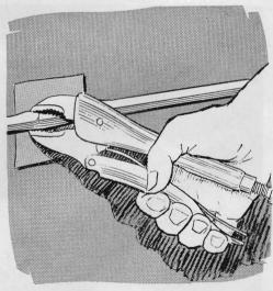
Dents in chrome molding on car doors or fenders can be removed easily. Use a plier wrench to squeeze the molding back to original shape, after inserting a small square piece of masking tape or thin cardboard between sheet metal and trim to protect paint.
