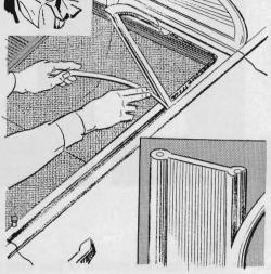
Stop window rattles the easy way. With the window down, push a piece of flat TV lead-in wire, 20 to 30 inches long, into the guide channel. The plastic coating will keep it in place. If the fit is too tight, shave a little bit of the plastic off one side of the wire.
