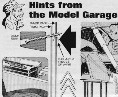
If armrest screw holes in a car door are stripped, you can make a repair by cutting and bending pieces of wire into a V shape, and hanging two or three of these in each hole. When the screw is refitted, its thread will have something to bite on.
