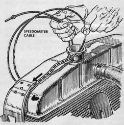
A clogged overflow pipe on the radiator can bring real trouble. It's important to keep the pipe open because pressurized cooling systems relieve excess pressure through it. You can clean it out easily by running a length of old speedometer cable through it.
