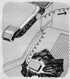
A simple parking-brake warning light can be made with a magnetic reed switch and a magnet. Tape the magnet to the brake-pedal arm and install the switch so it's actuated when the brake is applied. Fit a warning light on the dash and wire it in series.
