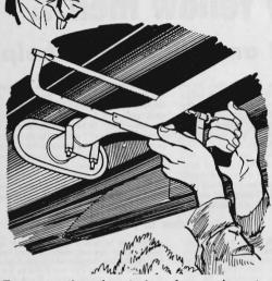
To remove the exhaust pipe when you're cutting loose a muffler, do it this easy way. Turn a hacksaw upside down and hold it around the pipe; then insert the blade with the edge toward the frame. This gives you more leverage, and the saw will bind less.
