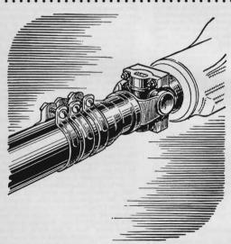
Vibrations in a car can sometimes be traced to an out-of-balance propeller shaft. If it's a slight eccentricity or out-of-roundness, you can fix it with a couple of hose clamps tightened around the shaft, with the screws positioned opposite the eccentricity.
