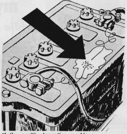
If the positive/negative markings are worn off your battery posts, you can identify the terminals by dipping the ends of two wires connected to the terminals into a small pool of electrolyte. Watch for bubbles from one wire-that's the negative one.
