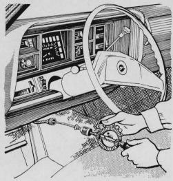
If you have trouble inserting a new speedometer cable, or a newly greased cable, into the outer casing, try this method: After feeding in the transmission end of the cable, chuck the instrument end in a hand drill and turn the cable as you push it in.
