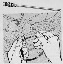
Spark-testing with an ordinary screwdriver is difficult when the plug terminals are sheathed in rubber. Make this handy spark tester by breaking an old spark plug apart for the core. Snap the cap onto a terminal and the core is exposed for testing.
