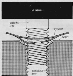
Stripped threads on the air-cleaner hold-down stud can be fixed by installing a 5/16-inch flat speed nut on the stud, as shown, after removing the carburetor top and countersinking the stud hole. The stud will then screw in tight and hold the air cleaner firmly.
