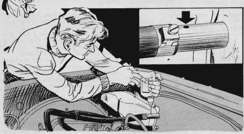
To bleed an air-bound heater element it isn't necessary to drain the car radiator. You can do the job in a simpler way by pulling the top heater hose almost free of the heater connector tube and drilling a 1/16- or ½-inch-diameter hole (arrow) in the top of the tube
