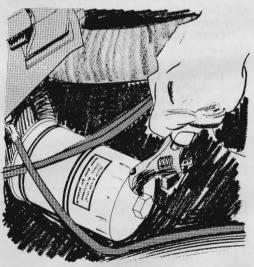
When changing oil and oil filters on some engines, the oil pump may lose its prime and fail to pick up. Here is an easy remedy: Loosen the filter a little and start the engine. This will make the pump pick up the oil. Stop the engine and retighten the filter.
