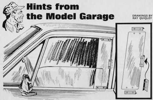
Rain and drafts when a door window is partly open can give you trouble on a '65 Plymouth. This happens because of an inward slant in the glass as it is lowered or raised. To fix it, get a piece of Plexiglas and cut it, as above, following a cardboard pattern. Make four 2½"-by-¾" angle
