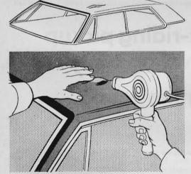
Air bubbles in a vinyl-covered roof can be removed by heating the vinyl in the bubble area with a heat lamp or a Master HeatGun (available at power-tool stores). The loose vinyl shrinks when heated lightly and can then be pressed down with your hand.
