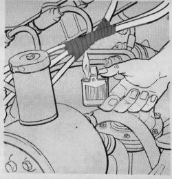
Removing electrician's insulating tape wrapped around a splice on auto-lighting wires or wiring harnesses can be difficult, especially if the splice is in a cramped place. It will soften up and come off easily if you pass a match or lighter flame across the tape a few times.
