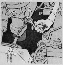
Getting a good grip on a bolt or nut with a pair of pliers is difficult if the fastener is where you can only reach it with one hand. The solution is to place a wide rubber band across the handles, holding them together. This way, you can turn your hand to get a new grip.
