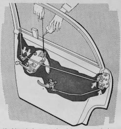
If side windows are hard to open and close, the mechanism may need oiling. Lower the glass all the way, wedge it to one side, and insert a stiff wire down to the mechanism. Oil deposited on the wire will follow it right to the desired part. This works with door locks, too.
