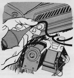
Check valves in the electric windshield-washer pump motor sometimes get clogged. There is no need for you to take the pump apart-just disconnect one of the water-outlet hoses and the inlet hose. Fill a syringe with fairly warm water and force it into the tube via the inlet tube. This will clean out the check valves.
