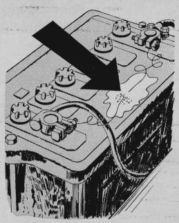
Positive or negative? Here's a fast way to identify the terminals of your battery if the markings are worn off: Dip the ends of two wires connected to the terminals into a small pool of electrolyte. Bubbles will form at the negative lead's tip.
