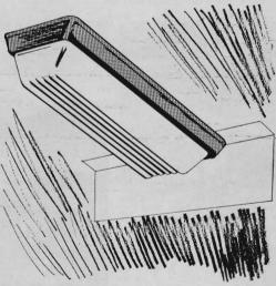
A car's dome light can be used at night by back-seat passengers without disturbing the driver, if you install a cardboard shield. Wedge the bent edge between the light and the headliner. Position it so it casts a shadow over the driver's area.
