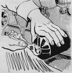
When installing an oil-filter element in a top-cover or shell-type casing, be sure to hold the cover or shell tightly in place while tightening the center bolt. If you keep the shell from turning, the gasket will seal and assure freedom from leaks.
