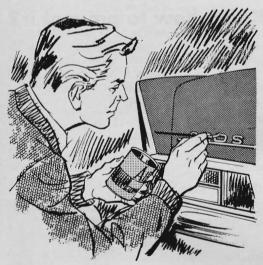
To mask chromium emblems or other trim before painting, put some grease on your finger or use a small brush to cover the parts you don't want painted. After spraying, wipe the grease off. Clean the area with a detergent when the paint dries.
