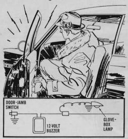
A headlight reminder could save you a dead battery. Put in an additional door-jamb switch at driver's side, connect it to a 12-volt buzzer and in turn to the glove-box lamp (hot only when headlights are on). Open the door and the buzzer sounds.
