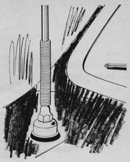
A broken radio-antenna staff can be neatly repaired at little cost by piecing the ends together with a heavy coil spring. Use a plated spring about 5" long that will fit tightly over the ends of the broken antenna after they're filed smooth.
