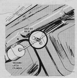
Safeguard a vacuum-operated trunk release by installing a cutoff valve in the vacuum line. This will keep a thief from opening the trunk by working the hose under the instrument panel. One of those valves used to aerate fish aquariums works fine.
