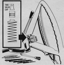
When the horn contact on '59-60 Thunderbirds becomes badly worn, a permanent fix can be made by cutting the tip off a metal tire-valve cap, and removing the rubber insert. Smooth off the cut and slip the cap over the contact-spring end to extend it.
