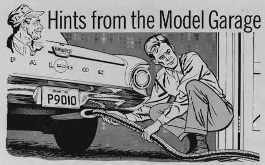
Make your garage a safe place to work in when you tune up your car's engine by venting deadly carbon monoxide exhaust gases outside with a snaking tailpipe extension. A length of flexible steel tubing or an old vacuum-cleaner hose will do the job. Be sure the diameter of the extension is such that it makes a leak-free fit around the tailpipe. Run the free hose end outdoors—and away from windows and siding: Exhaust fumes can discolor painted woodwork and corrode exposed metal surfaces.
