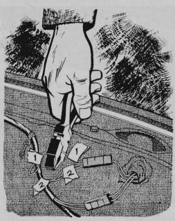
When removing electrical equipment, don't cut any wires until you've stuck small masking-tape "flags" on either side of the cut. Label each pair with the same number. There will be no confusion when it's time to reconnect; just match up the numbers.
