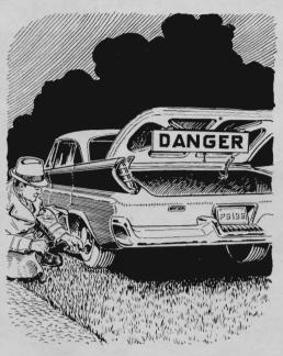
A hinged reflective sign hanging from the trunk lid can save your life when you make emergency repairs at night. It's made of a 4'-by-8" piece of ¼" plywood with red reflecting-tape letters. A cupboard door catch holds it up against lid till needed.
