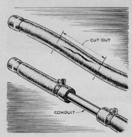
Burst radiator hose is easily repaired with a piece of thin-wall conduit and two hose clamps. Use ½" conduit for conventional ½" hose. This splice also can be used to make a permanent repair at any point where the hose rubs and wears fast.
