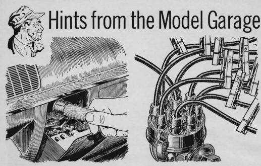
Cigarette-lighter problems often are caused by a poor ground between lighter and dash. To tighten the electrical connection, taper one end of a 6" piece of broomstick, wrap in emery paper for a snug fit in the lighter casing, and twist the casing.
