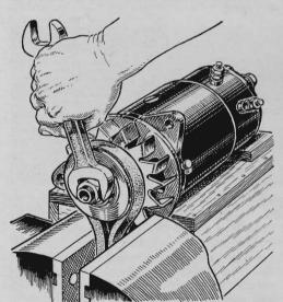
To loosen the nut on a generator, wrap an old fan belt around the pulley as tightly as possible. Then squeeze the belt in a vise. This will hold the generator securely and allow you to remove the nut without danger of damaging fragile parts.
