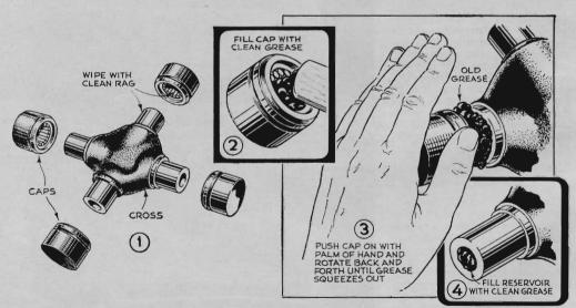
Packing a universal joint is easy if you follow this procedure: When the joint is disassembled, wipe out as much of the dirty grease in the cap and cross as you can reach with a clean rag. Then fill the cup with clean grease and force it back on the cross shaft, twisting it back and forth with the palm of your hand. The dirty grease will be forced out and can be wiped away. Repeat until the grease comes out clean. Now you can fill the reservoir and reassemble the universal joint.
