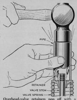
Overhead-valve retainers pop off with a minimum of fuss if you force them out with a piece of pipe. Slip the pipe over the valve stem onto the retainer washer. Strike the pipe a solid blow with a hammer. The retainers will jump out inside the pipe.
