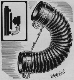
Installing a flexible lower radiator hose isn't easy when working room is limited. Try preshaping the hose into a U and fastening the ends with wire. Position hose and loosen the wire. This releases the hose, which forces itself into place.
