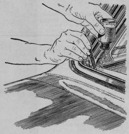
Silence loose, squeaky windshields and rear windows with a little ordinary talcum powder. Run a nail file around the rubber gasket that holds the glass in place. As you pry the rubber away, sprinkle the powder between the gasket and the glass,
