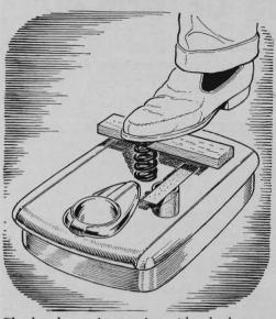
Check valve-spring tension with a bathroom scale. Cut cardboard tube to length specified for compressed spring. Lay cardboard strip over tube, and block of wood over spring. Step on wood. When the strip starts to tip, take a reading on the scale.
