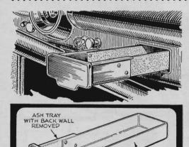
Use your pull-out ash tray as a storage box if you're a nonsmoker. Remove the back wall and extend the length of the tray with sheet metal. You will then have a handy storage compartment for a pencil, pen, comb, tire gauge, and other small items.
