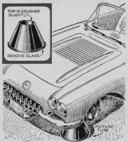
An inexpensive axle and frame stand can be had from your TV repairman; just ask him for a burned-out picture tube. Have the glass removed (let him do this). The top of the metal cone will crush slightly in use; this keeps the car from slipping off.
