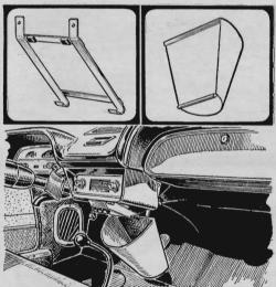
Install a litter basket in your Corvair under the radio. A cross-braced bracket hangs on screws in back of the radio. A ¼" dowel glued to the bottom of the basket fits curved bracket ends. Two magnets on the bracket hold a metal strip at top.
