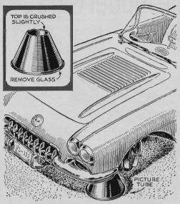
An inexpensive axle and frame stand can be had from your TV repairman; just ask him for a burned-out picture tube. Have the glass removed (let him do this). The top of the metal cone will crush slightly in use; this keeps the car from slipping off.
