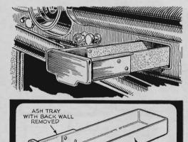
Use your pull-out ash tray as a storage box if you're a nonsmoker. Remove the back wall and extend the length of the tray with sheet metal. You will then have a handy storage compartment for a pencil, pen, comb, tire gauge, and other small items.
