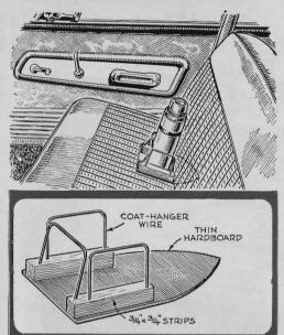
A wire holder for your thermos bottle will keep it from tipping when you turn or stop quickly. Cut the flatiron-shaped base from hardboard. Tack and glue wood strips to it and drill them to accept coat-hanger wire. The base slips under the front seat back.
