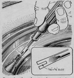
Removing the valve stem from a tire is an easy job with this homemade valve tool. Cut a 16" slot in the tip of a thin-bladed screwdriver with a hacksaw and file. You may have to grind down the edges of the blade so it will fit inside the valve.
